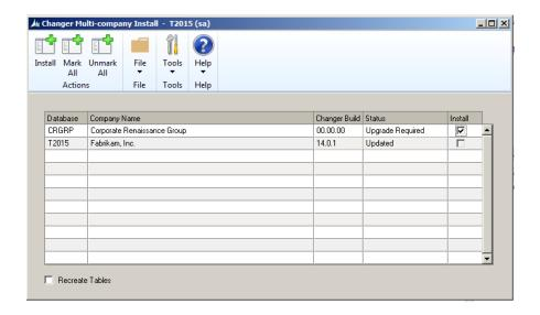
Select the companies you wish to install Changer on by clicking the check-box in the 'Install' column. All the companies can be marked or un-marked by using the 'Mark All' and 'Unmark All' buttons respectively. Once the companies are selected for installation, click the Install button to start the installation. After successful installation, the status will change to 'Updated' for each company and the Changer build will show the latest Changer build.
